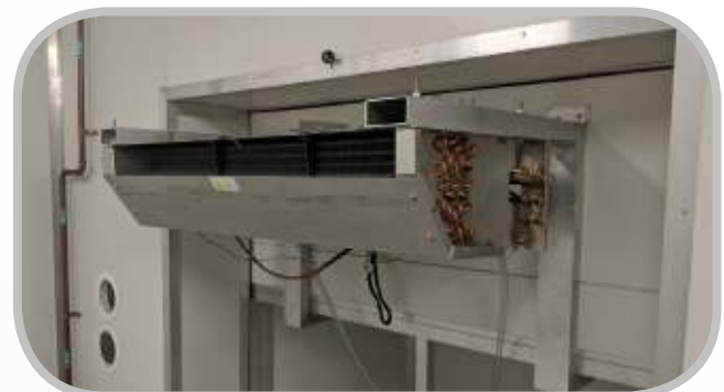
Image 3: Citimax 700 evaporator unit in thermal test chamber
