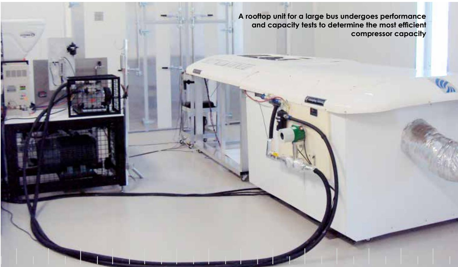
A rooftop unit for a large bus undergoes performance and capacity tests to determine the most efficient compressor capacity
